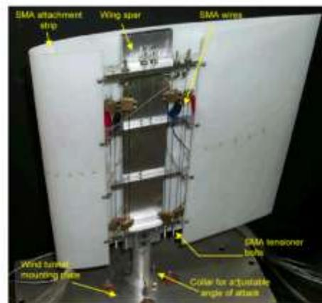
Figure 2-22 Reconfigurable Wing Wind Tunnel Model
