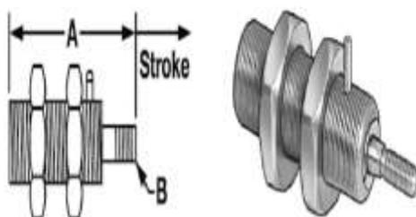
Figure 3-2 Miniature threaded-body air cylinder
