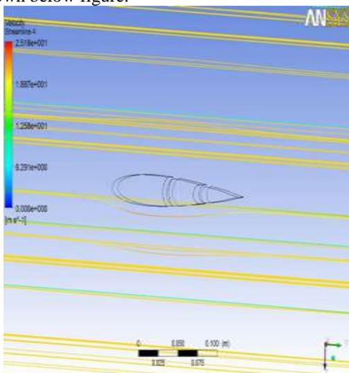
Fig5.3.5: Stream line Flow along the VCW model
