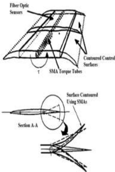
Figure 2-23 Smart Wing Model
