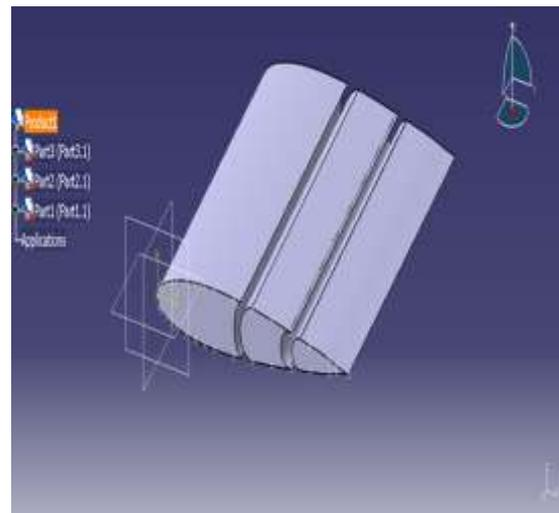
Fig5.4.6: catia model of structure assembled of multi-section variable wing
