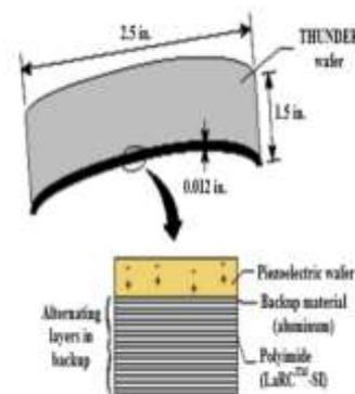
Figure 2-18 Enlarged Isometric View of THUNDER Actuator
