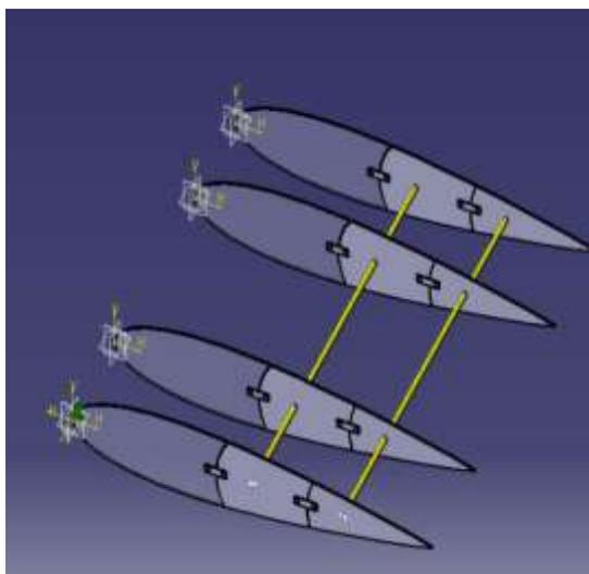
Fig5.4.5: Catia model of structure assembly of Multi-Section Wing
