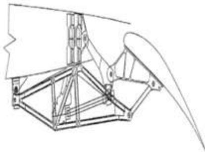
Figure 2-9 Four-Bar linkage system used to support and actuate outboard single-slotted flap on B777
