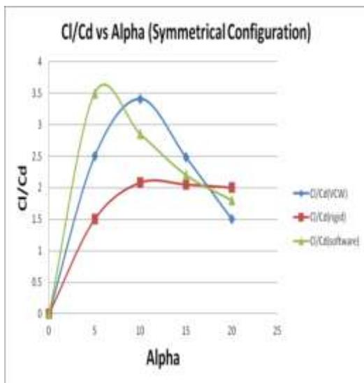
Fig5.5.3: Graph of Cl/Cd vs. Alpha
