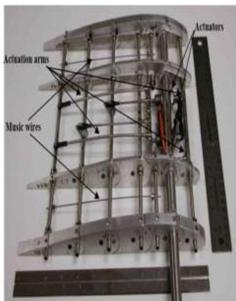
Figure 3-11 Wing structures Assembly
