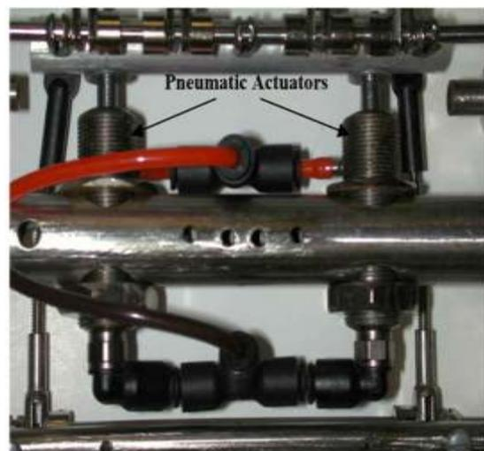
Figure 3-9 Actuators installed inside the main spar
