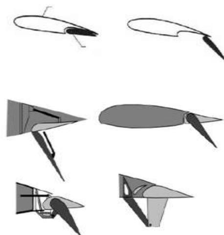
Figure 2-4 Closed and Opened Positions of Fowler Flap
