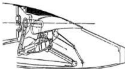
Figure 2-10 Link-Track mechanism used to support and actuate single-slotted flap on A320
