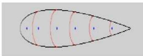
Figure 3-1 Cross-Section Drawing of the Multi-Section Variable Camber Wing
